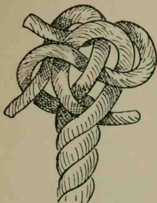
FIG. 121 A.—Making double crown.
